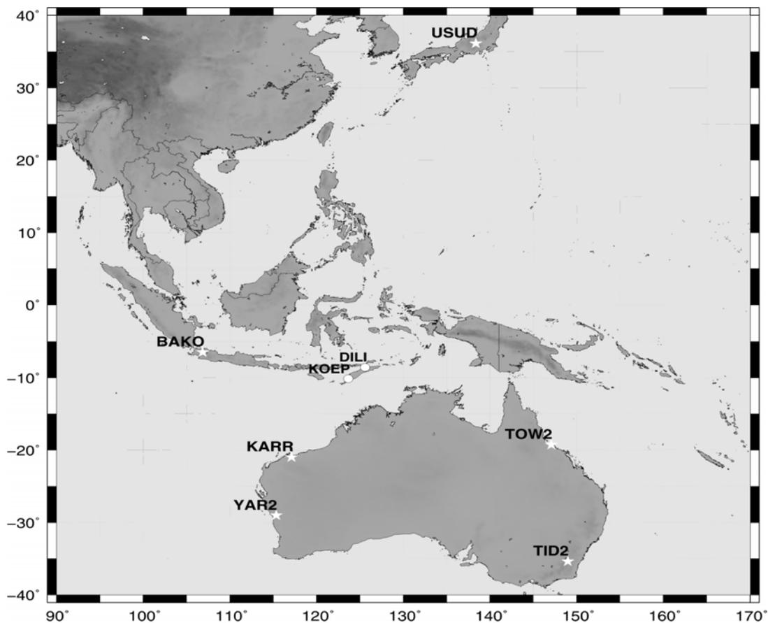
Figure 2 – IGS stations (white stars) used to map the CBDRF network into ITRF2000. The continuously-operating stations (white circles) in Timor are also shown.
